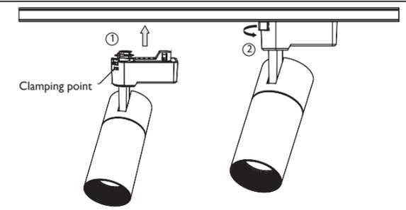
Put the track joint into the track, and rotate the track head clip past the clamping point to ensure that the conductor is in full contact.
