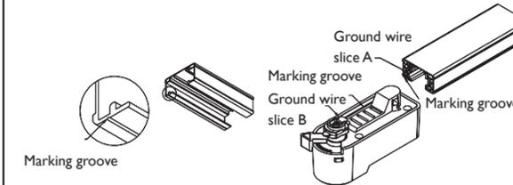
When installing, please first match the marking slot on the track joint to the marking slot on the track strip, and do not reverse install.
