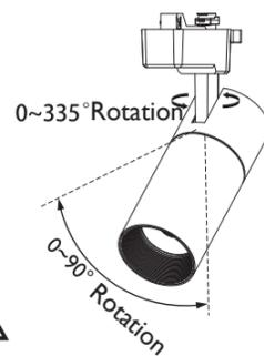
Only adjust the lighting angle when the power is off.
