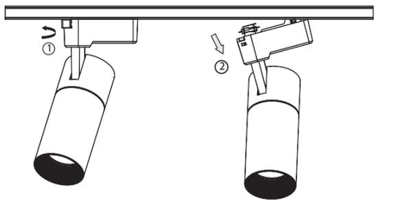
Rotate the track head clip to the other end of the clip point and tilt the lamp according to the drawing until the track is pulled out.
